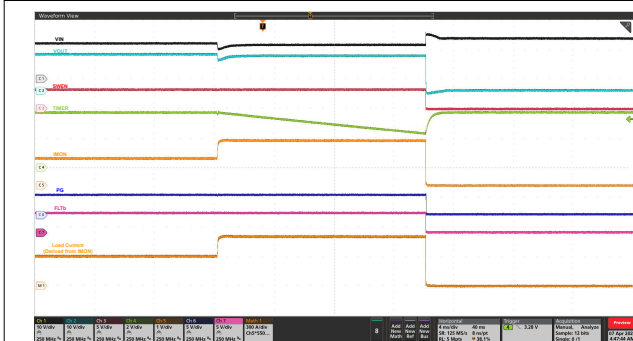
Figure 9-8. Circuit-Breaker Response: V_{IN} = 12 V, C_{TIMER} = 22 nF, C_{LOAD} = 55 mF, R_{IMON} = 167 \Omega , R_{REF} = 40.2 k \Omega , and Load Current Stepped up From 300 A to 500 A for > 20 ms
