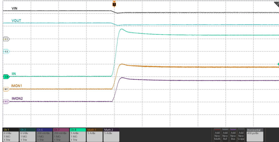
Figure 8-10. Parallel Devices Load Current During Steady State
