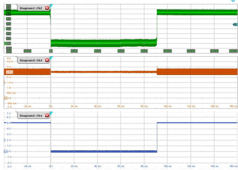
Ch2: Output voltage (1 V/div); Ch3: LED current (500 mA/div); Ch4: \overline{\text{FLT}} voltage (1 V/div); Time: 20 ms/div
