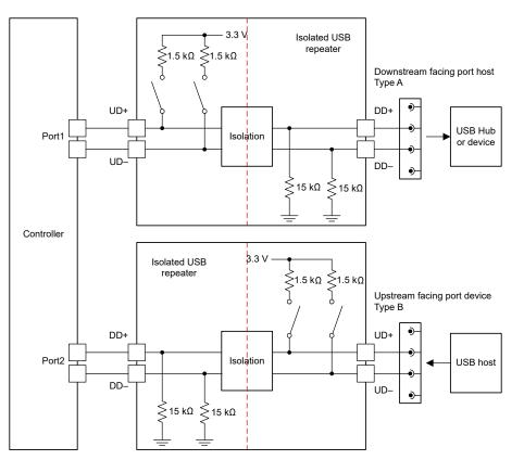
Figure 1. Traditional implementation offering dedicated host and peripheral ports with two isolated USB repeaters
