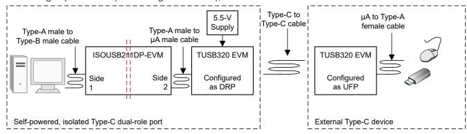
Figure 5. The ISOUSB211 and TUSB320 as a DRP connected to a USB Type-C device or peripheral
