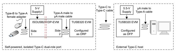
Figure 6. The ISOUSB211 and TUSB320 as a DRP connected to a USB Type-C host
