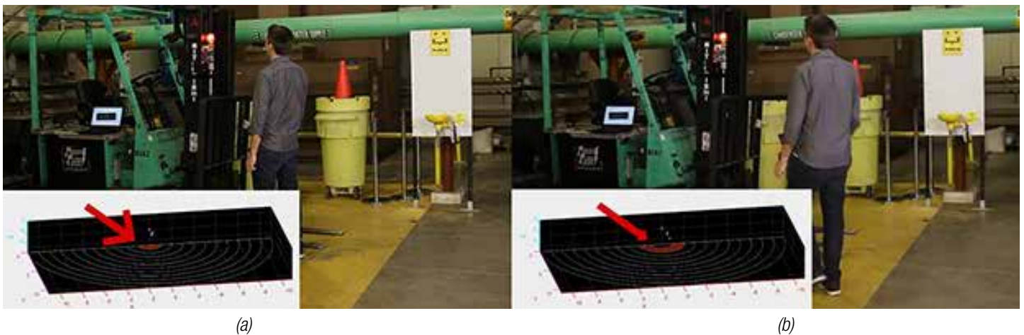
Figure 3. The danger sign triggers at 1 m when a person is walking slowly (a); and at 2 m when a person is walking fast (b).
