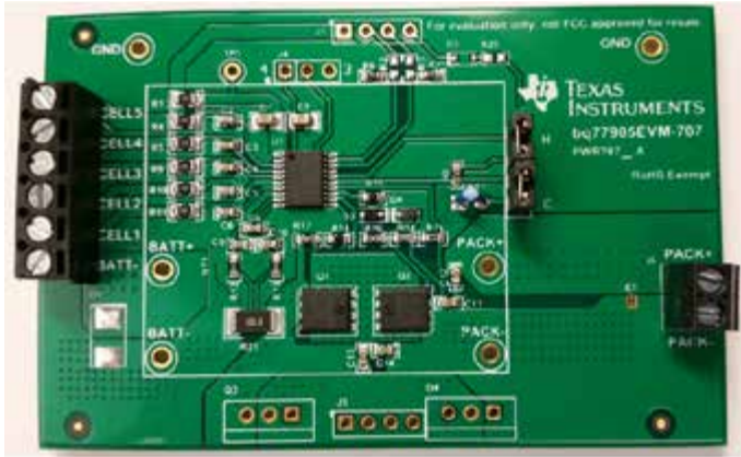
Figure 1. BQ77905 3S to 5S advanced stackable low-power battery protector EVM.
