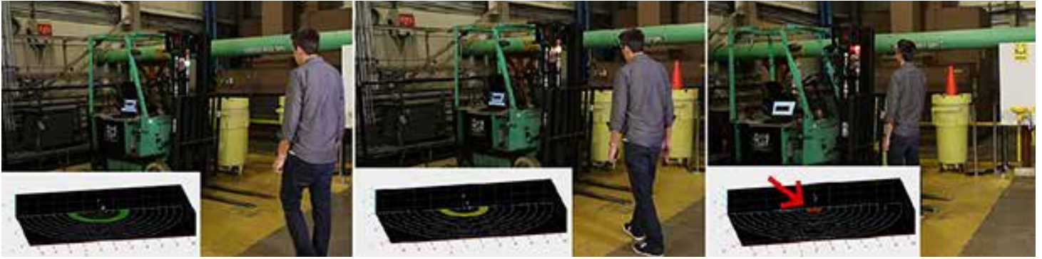
Figure 2. A person walks slowly past a machine and the danger signal flashes at 1 m.
