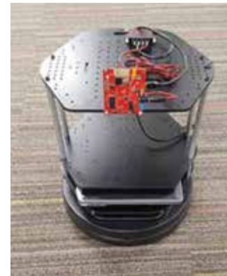
Figure 9. IWR1443 EVM mounted on a Turtlebot 2.
