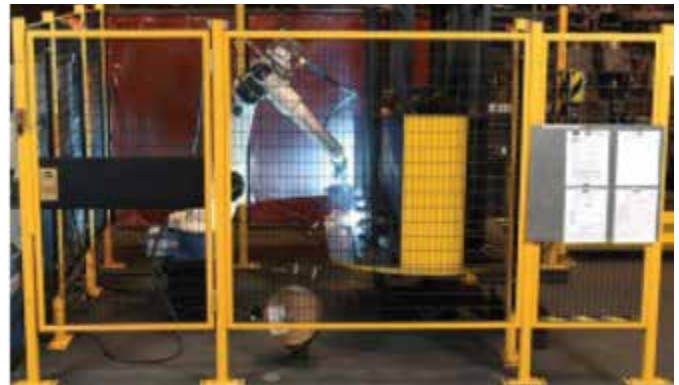
Figure 6. Robotic arm with a physical safety cage.
